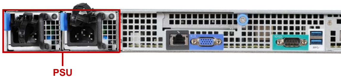
Figure 1-8. PSU to Mainboard Module Description
