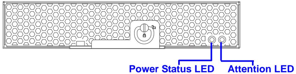
**Figure 1: Blade LED (front view shown)**
