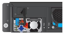
**2** Press the plug retainer and then pull the handle to slide the PSU away from the chassis.
