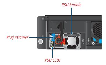
The AC power connector is a standard three-pronged connector. The switch automatically adjusts its power setting to any supply voltage in the range from 100~240 VAC at 50~60 Hz.
