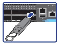
3 Repeat the above procedures to install additional QSFP28 modules.
