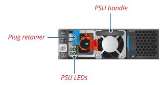
The AC power connector is a standard three-pronged connector. The switch automatically adjusts its power setting to any supply voltage in the range from 100~240 VAC at 50~60 Hz.
