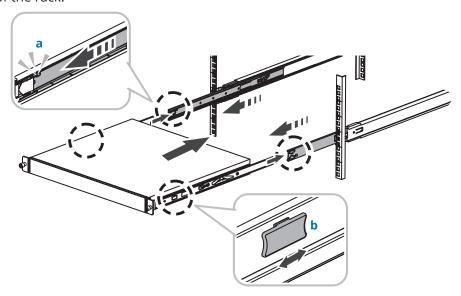
**6** Secure the switch to the rack using the screws.
