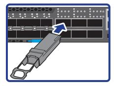
3 Repeat the above procedures to install additional QSFP28 modules.
