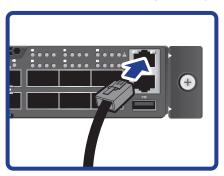
**2** Connect the other end of the Ethernet cable to a network.
