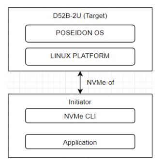
Figure 1 Target-client architecture of PoseidonOS
