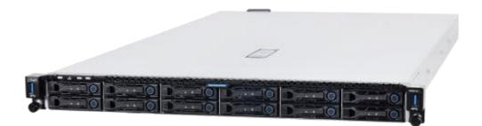
Figure 2 High density fast storage NVMe server
